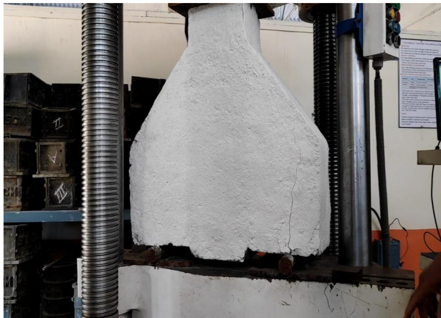
Fig.4. Testing of corbel on UTM
