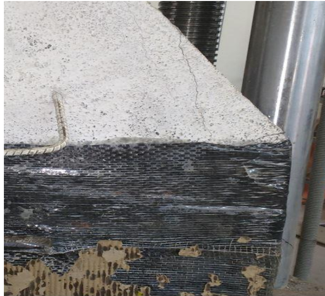
Fig.7. Crack developed for the horizontal wrapping at ultimate load
