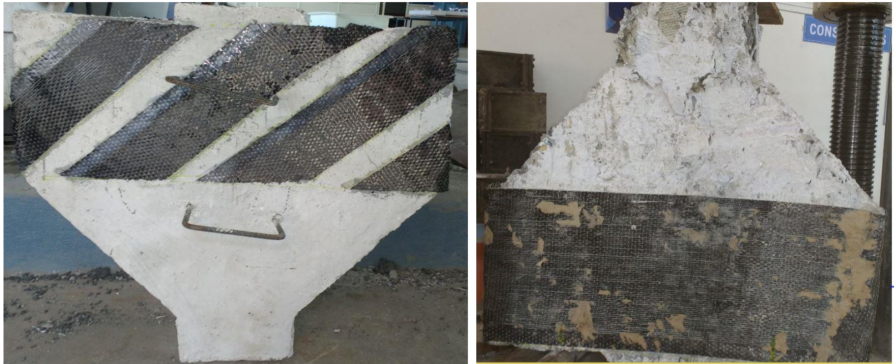
Fig.3. Inclined and horizontal pattern of confining of CFRP
