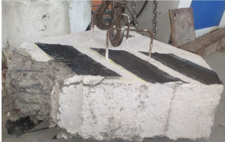
Fig.9. Peeling out of CFRP after crushing of concrete
